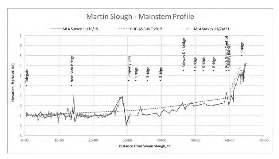
Figure 3. Mainstem channel profile showing the As-Built/Design Condition (Year 0), the Phase 2-4, Year 1 condition and the Phase 2 Year 3 condition. The two high spots in Phase 2 Year 1 at the Barn and Property line are still present in Year 3.
