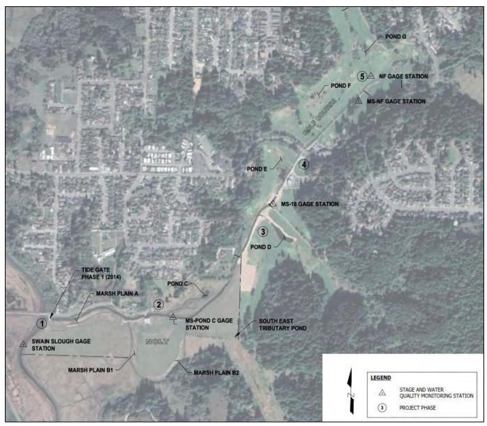
Figure 2. Overview of Phases 1 through 5, and location of stage and water quality monitoring stations (image from Google Earth, Oct. 2019).
